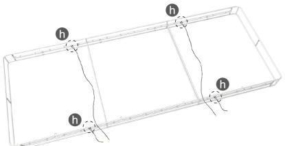
③ Connect those 2 adjacent LED light bars connected with Y-shaped connection wire, slightly adjust space between each LED light bar from 1" to 4".
