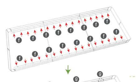
① Slide clips from LED light bars to align at holes of poles & press into.
